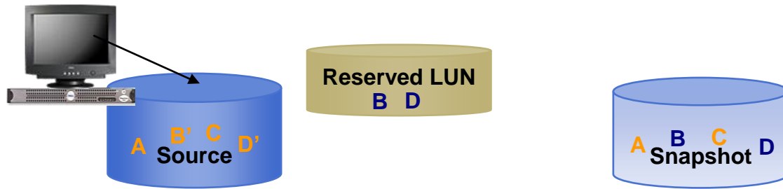
Figure 1. A SnapView snapshot as a composite of unchanged source data and data saved on the reserved LUN
